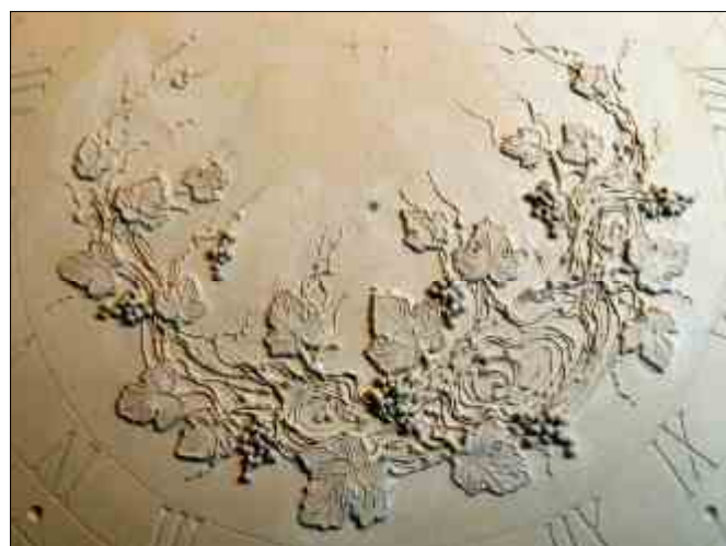
Fig. 4 (top). The last examination before turning the pottery into the porcelain dial.
