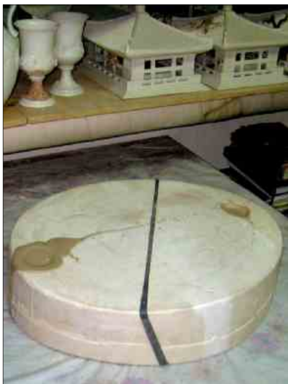
Fig. 1. Mould with two funnel-shaped holes.
